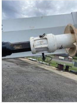
P103.2: Has the wrong pin in auger
